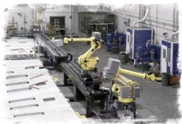
Figure 5: Northrop Grumman robotic facility in Palmdale CA applying AHFM material on B-2 parts
